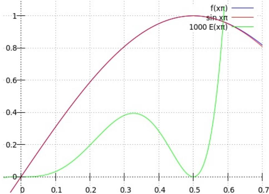
As the plot shows, we end up with a maximal error of about 0.04 %, 1/10 of what we got from  $f_0(x)$ . Explicitly we find the error maximum at
