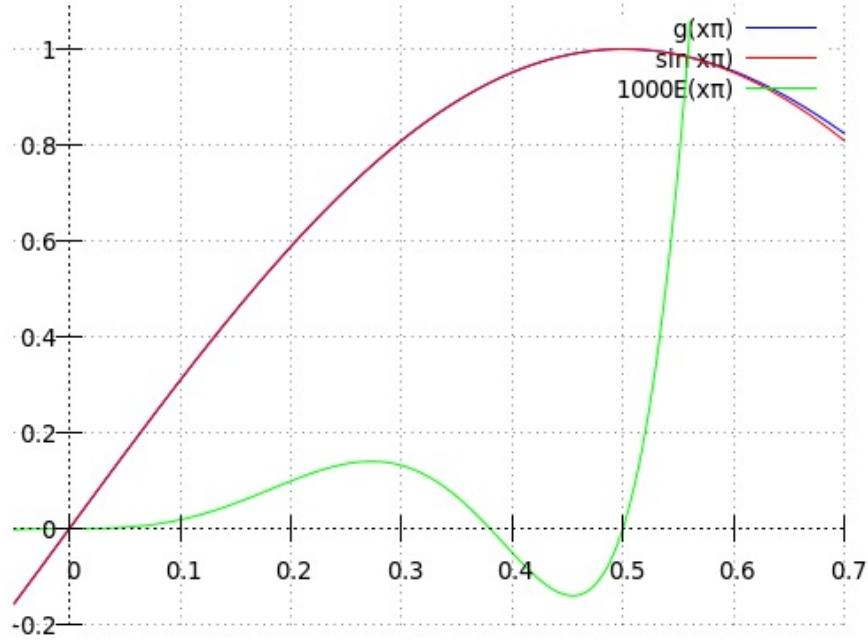
Requesting  $g'(0) = 1$  (as  $\sin' 0 = 1$ ) has automatically led to  $E'(0) = 0$ . So the error function starts very softly from  $x = 0$ . Can we achieve smaller absolute extrema by allowing the error to rise more sharply? This means dropping  $g'(0) = 1$ , so we are back to the full  $g(x)$  from equation (4), and to this list of requirements:
