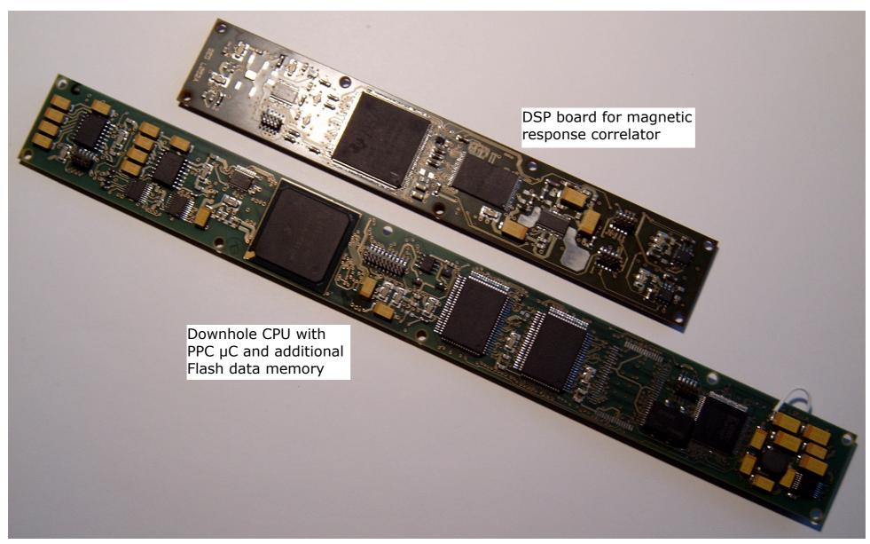
Two Boards for Inertial Well Bore Surveying Designed by **binär** industrie-informatik Bernd Kohler
